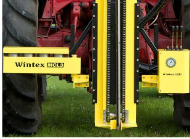
The **WINTEX MCL3** has its own hydraulic system and can be mounted on vehicles like John Deere Gators, pick-ups, ATVs and caterpillar vehicles.
