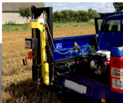
Can be delivered with different holding boxes which fit most of the commonly available sample boxes or with a soil box from which the sample can be filled directly into a soil bag.
