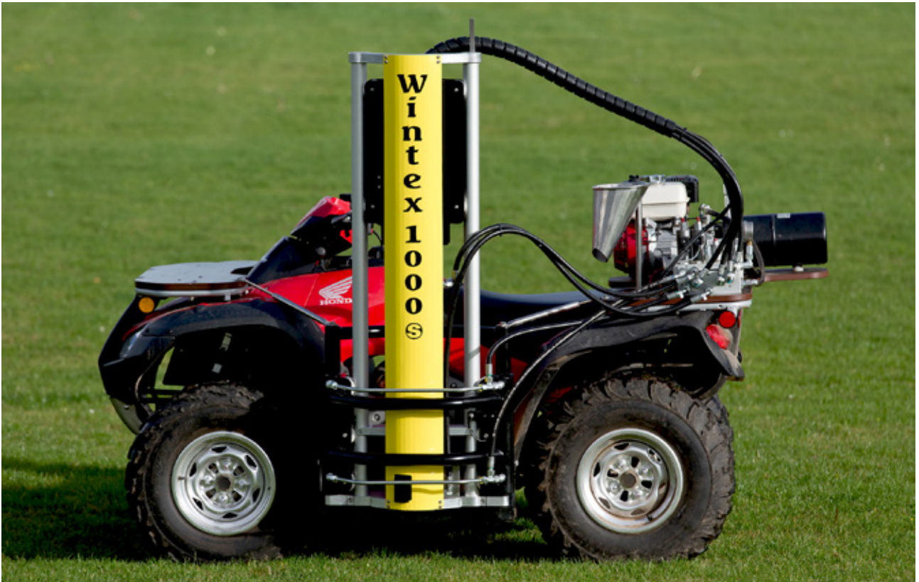
The Wintex 1000s can be mounted on many vehicles. Here it is mounted on a Honda ATV.
