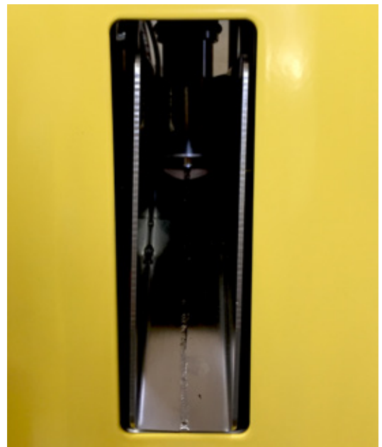
If the Wintex 3000 meets obstacles or is interrupted during soil sampling and therefore only takes a half sample, the sample will be discarded through this funnel and not be filled into the soil boxes.
