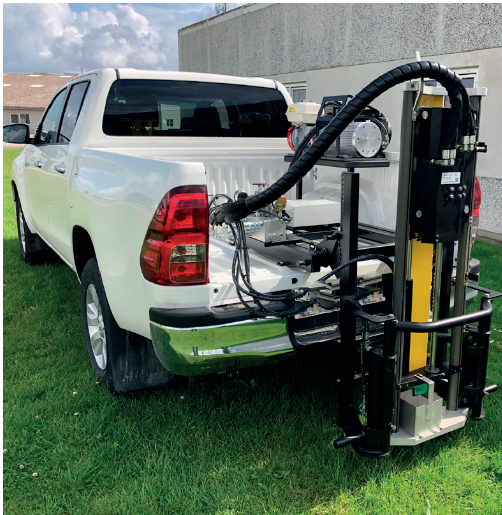
The WINTEX 1000s can be mounted on all vehicles including pick-ups, tractors and trailers.
