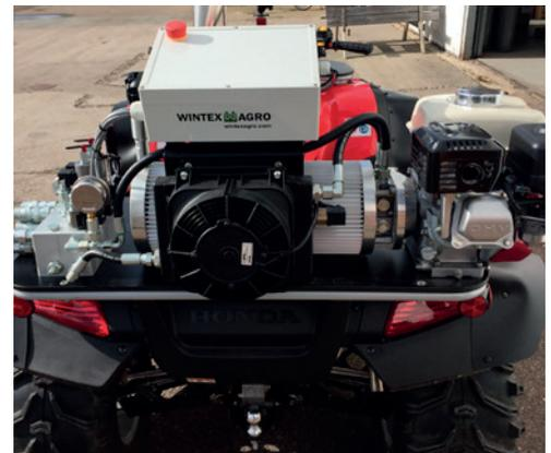
The custom-made oil tank is made of aluminum. It has a ribbed surface which means that its area is three times larger than a plain surface. Because of the aluminum and the ribbed surface the cooling capacity is 12 times higher than the cooling capacity of a traditional oil tank. This means that the tank ensures optimal cooling of the hydraulic oil.
