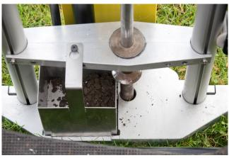
The collected soil is directly delivered into the soil box from which it can be filled in a box or a bag ready to be sent to the laboratory.
