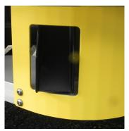
If the WINTEX 1000s meets obstacles or is interupted during the sampling proces and therefore takes an incomplete sample, the sample will be discarded through a funnel and will not be filled into the soil box.
