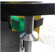
The scraper fits the inner diameter of the probe precisely, and the scraper blades ensure that the probe is emptied fully before going into the gound again.
