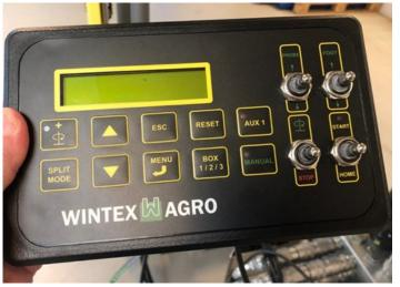
All fuctions can be carried out from the control system. Pre-settings like the depth and thje amount of sticks per sample can quickly and easily be entered into the the control system.
