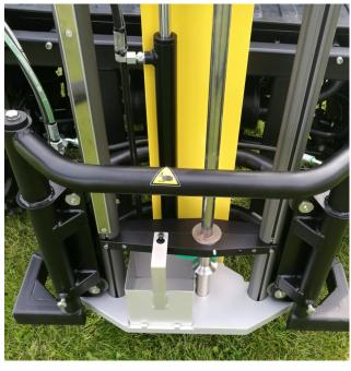
Mounting the **WINTEX 1000s** on a reversed frame ensures easy access to the soil box.
