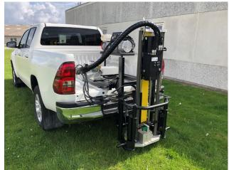
The **WINTEX 1000s** can be mounted on a wide range of carrier vehicles, for example ATVs, UTVs, tractors, pick-ups, low tonnage vans and trailers.
