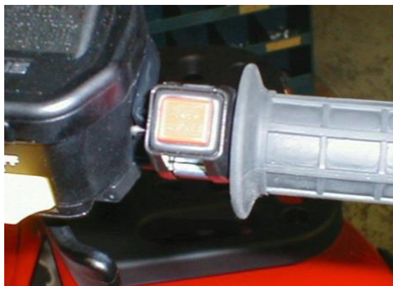
The start switch mounted on the right side of the handlebar – here on a Honda ATV
