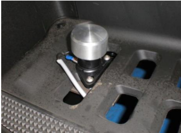
Foot contact mounted on a Honda TRX680
