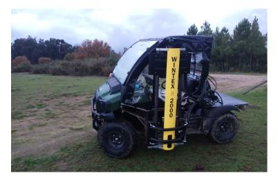
Sample depth: 0-60 cm Diameter probe: 15 Samples / hour: Sticks / hour: 225 Volume / sample at a densitiy 1:1 1.5, 2.0 or 2.5 g per cm -
