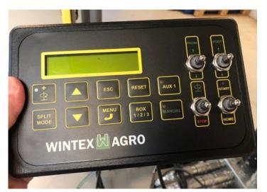
All actions can be carried out from the control system. Pre-settings like the depth, sticks and layers per sample as well as choosing the soil box can quickly and easily be entered into the the control system.
