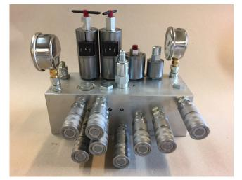
All functions are conducted by the custom-made distribution block. The hydraulic system has a simple construction which makes maintenance easy and uncomplicated.
