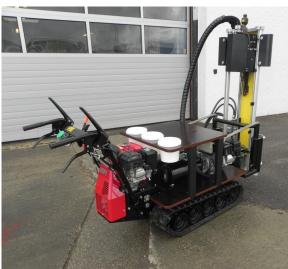
The **WINTEX 2000** can be mounted on a wide range of carrier vehicles, for example ATVs, UTVs, tractors, pick-ups, low tonnage vans and trailers.
