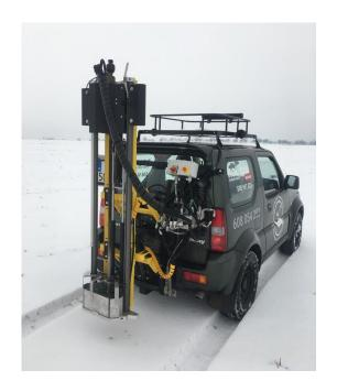
The WINTEX 3000 can be mounted on a wide range of carrier vehicles, for example ATVs, UTVs, tractors, pick-ups, low tonnage vans and trailers.
