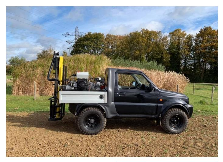
The **WINTEX 3000** is an efficient and strong automatic soil sampler. It is user-friendly, easy to use and requires only minimum maintenance. All functions are comfortably carried out from the driver's seat.
