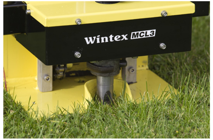
The probe goes into the ground by the means of a high-frequency hammer.
