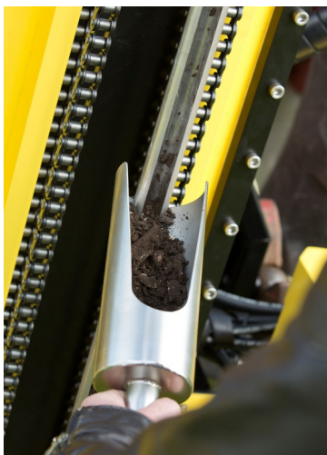
The soil is removed from the probe and filled into the soil bins with a sampling scoop and a scraper.
