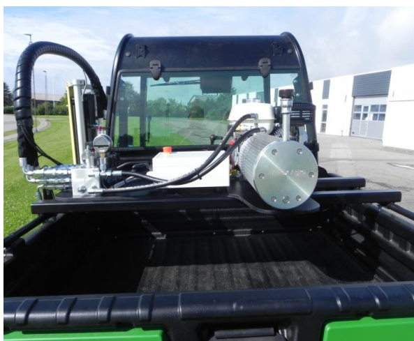
Oil pump and Honda GX 200 motor on a John Deere 855D
