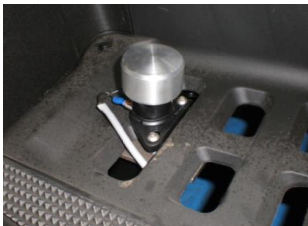
Foot contact mounted on a Honda TRX680
