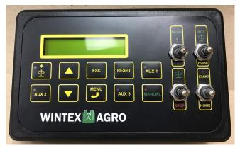
All functions can be carried out from the control system. Presettings like the depth and the number of sticks for each sample can quickly and easily be entered into the the control system.
