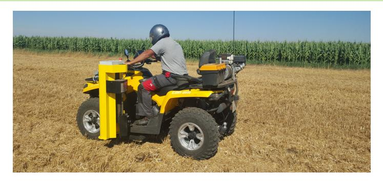
The **WINTEX 1000** is an efficient and strong automatic soil sampler for soil samples up to 25 cm. It is user-friendly, requires only minimum maintenance and is easy to use. All functions are comfortably carried out from the driver's seat.
