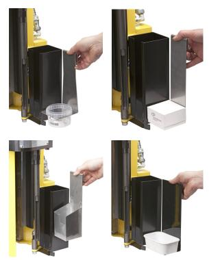
The **WINTEX 1000** is available with different holding boxes which fit the most commonly used sample boxes or with a holding box from which the sample can be filled directly into a soil bag.
