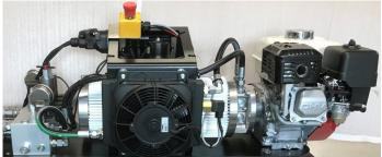
The custom-made oil tank is made of aluminum. It has a ribbed surface which means that the area of the oil tank is three times larger than a plain surface. Because of the aluminum and the ribbed surface the cooling capacity is 12 times higher than the cooling capacity of a traditional oil tank, ensuring optimal cooling of the hydraulic oil.
