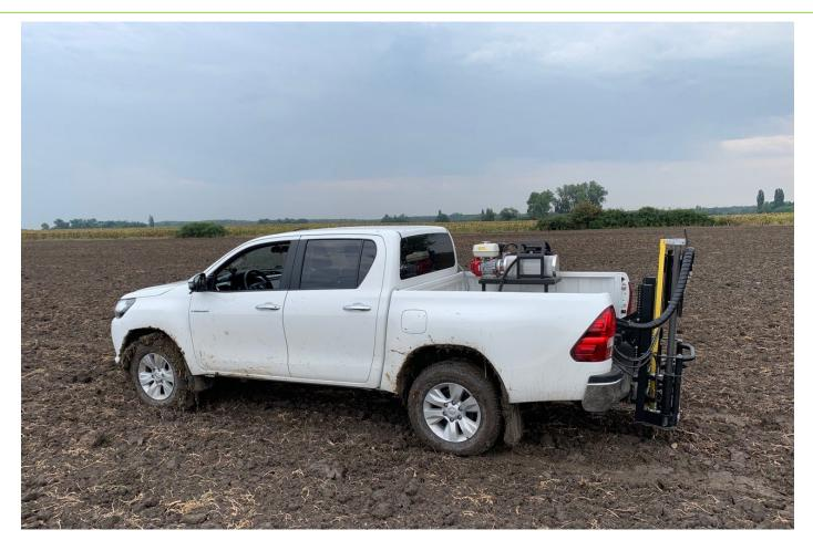
The **WINTEX 1000s** is an efficient and strong automatic soil sampler. It is user-friendly, easy to use and requires only minimum maintenance. All functions are comfortably carried out from the driver's seat.
