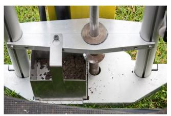
The collected soil is directly delivered into the soil box from which it can be filled in a box or a bag ready to be sent to the laboratory.
