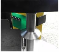
The scraper fits the inner diameter of the probe precisely, and the scraper blades ensure that the probe is emptied fully before going into the gound again.
