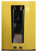
If the **WINTEX 3000** meets obstacles or is interupted during the sampling proces and therefore takes an incomplete sample, the sample will be discarded through a funnel and will not be filled into the soil boxes.
