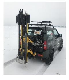
The **WINTEX 3000** can be mounted on a wide range of carrier vehicles for example UTVs, tractors, pick-ups, low tonnage vans and trailers.
