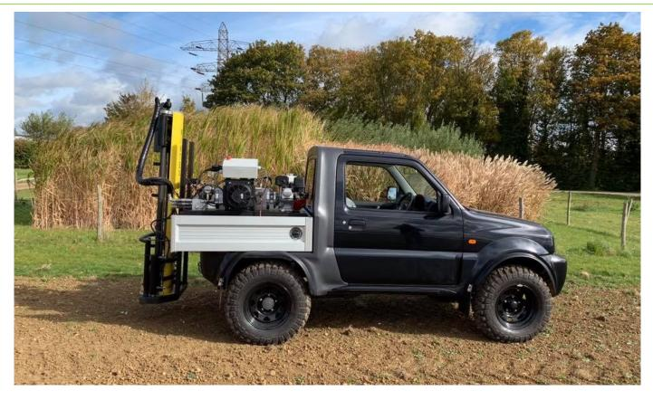
The **WINTEX 3000** is an efficient and strong automatic soil sampler. It is user-friendly, easy to use and requires only minimum maintenance. All functions are comfortably carried out from the driver's seat.
