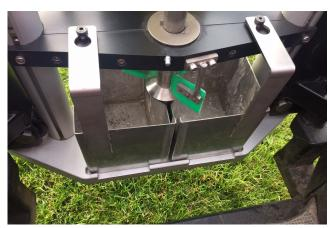
Soil from different layers is automatically filled into the soil boxes. Dividing the samples is conducted with close accuracy.
