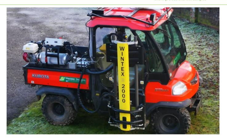
The **WINTEX 2000** is an efficient and strong automatic soil sampler. It is user-friendly, easy to use and requires only minimum maintenance. All functions are comfortably carried out from the driver's seat.
