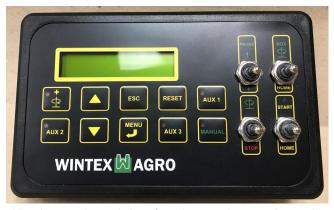
All actions can be carried out from the control system. Pre-settings like the depth, sticks and layers per sample as well as choosing the soil box can quickly and easily be entered into the the control system.
