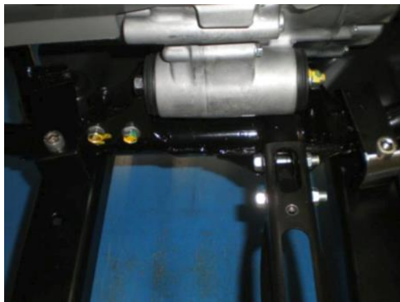
Left side - showing where the angle brackets are mounted
